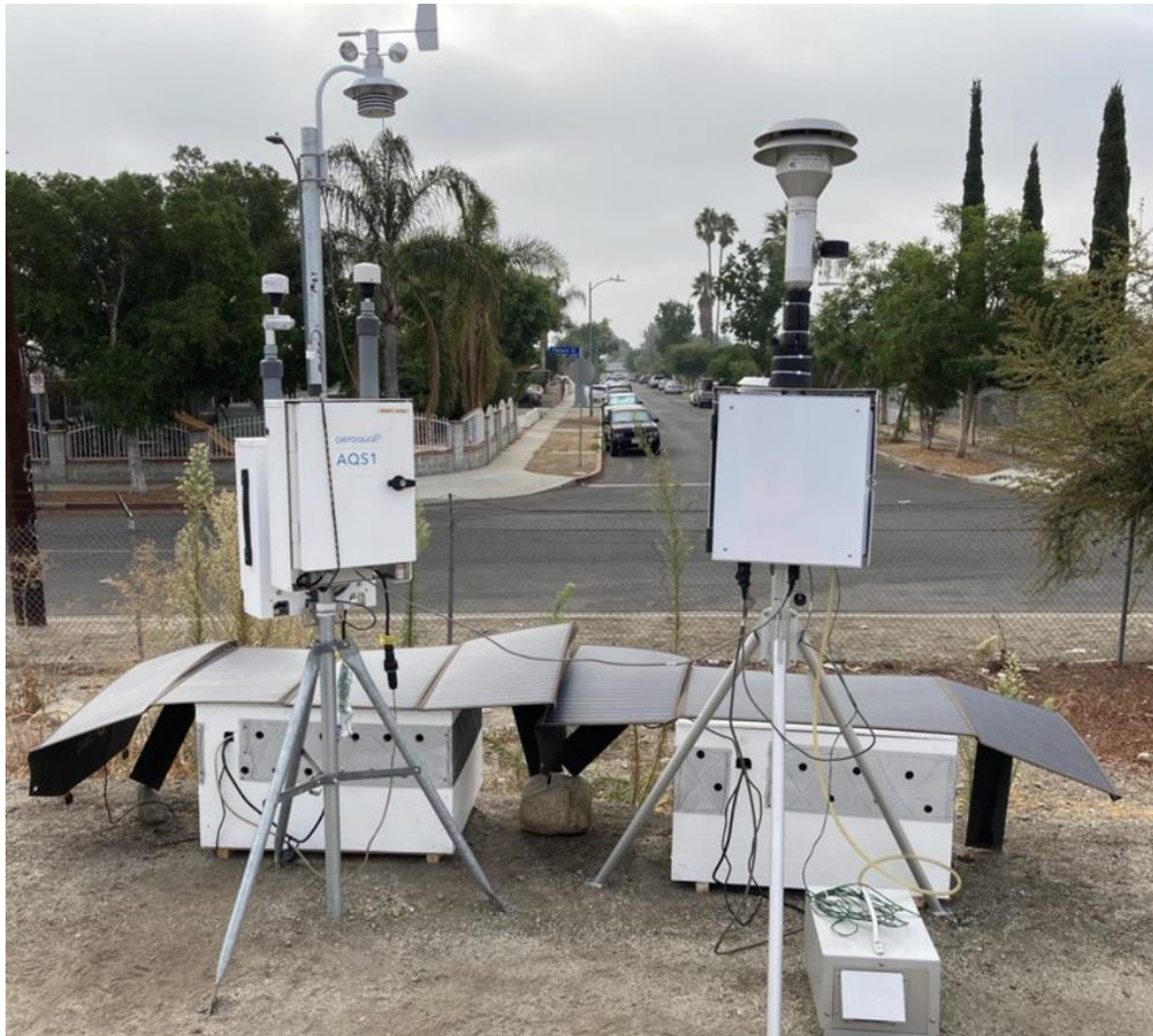
Figure 1. Background monitoring and field calibration set up including AQS-1, Dust Sentry, and EBAM+.
