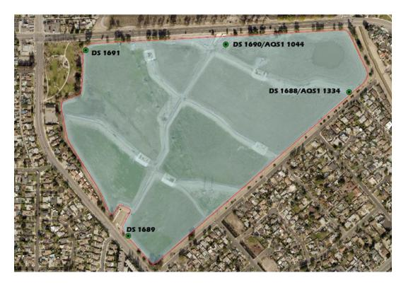
Figure 1. Pacoima Spreading Grounds air monitoring stations for the Southern site. DS: Dust Sentry.
