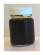
Typical Pyrolysis Oil HHV ~ 16-19MJ/kg 28-40% oxygen
